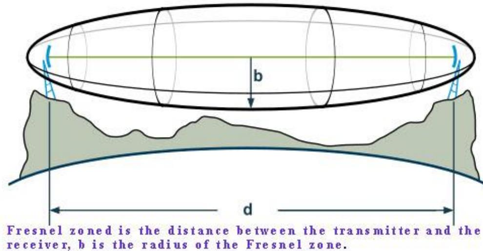
The max diameter of the Fresnel zone corresponds to the max height and width of the Capture Zone. The Capture Zone is the area the receiving antennas has to be in to receive the signal. Very useful when building arrays or using multiple antennas for MIMO.
