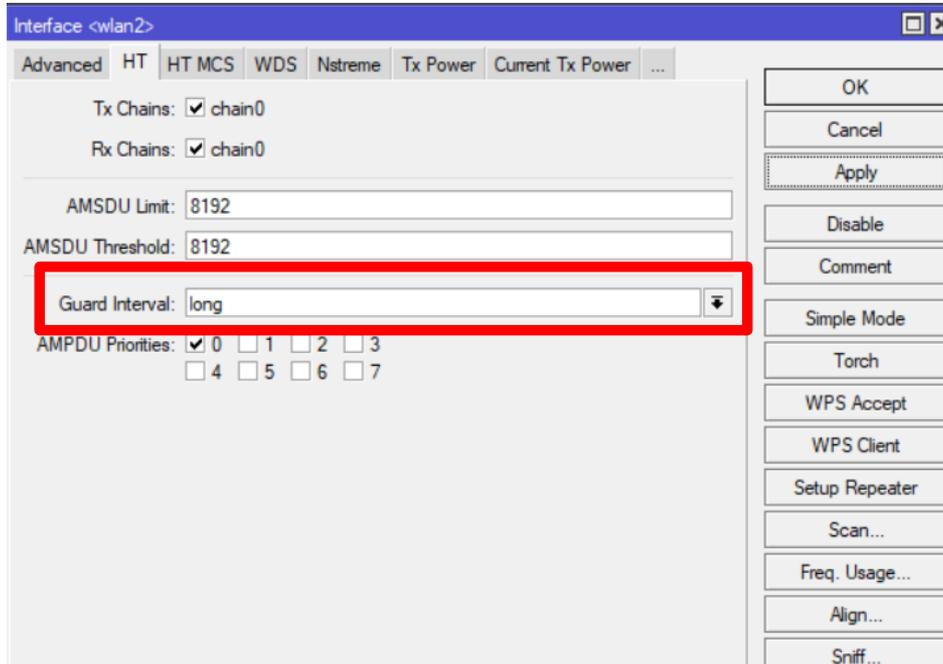
Setting the guard interval to long can result in fewer DFS choices for the radios and ultimately improve long term performance. This applies to both indoor and outdoor links. Don't be greedy!
