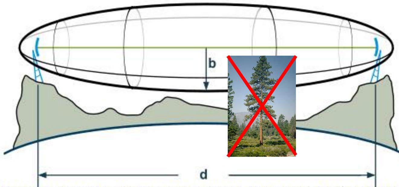
Fresnel zone is the distance between the transmitter and the receiver,  $b$  is the radius of the Fresnel zone.
